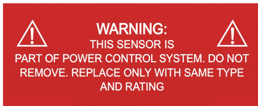
Figure 9 – PCS sensor warning label. Apply at the panel where the CTs are installed.
