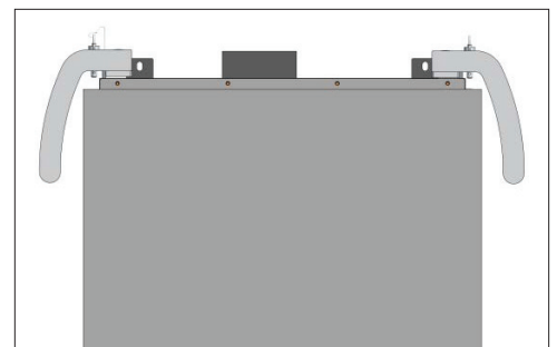
Fig 5 Grip rails sit at the front for a balanced team lift
