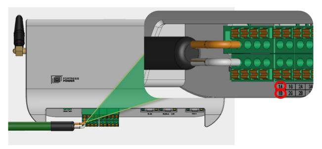
When setting up the Guardian with a Fortress Power Envy inverter, use the provided tworow, four-column connector to wire into the Guardian's communication port. For proper connection, refer to the cable pinout: connect the Orange wire to RS485 1A and the Orange/White wire to RS485 1B on the Guardian.
