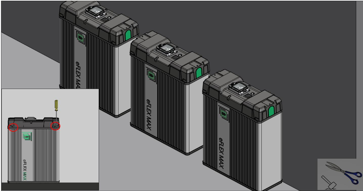
2. Connect the Battery-Battery Communication Cables. Follow the Downlink-Uplink sequence. Connect the Electrical cables using a torque socket wrench. The correct torque specification is **7.0 - 7.7 Nm (5.1 - 5.7 ft-lb)**.
