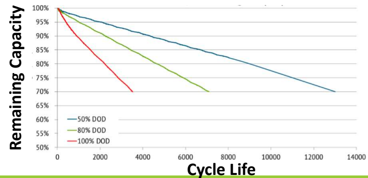
LFP Cycle Life in Relation to Depth of Discharge (DoD)
