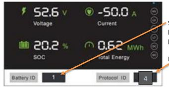
Set the battery ID to sequential numbers on each battery (1, 2, 3, 4, ... number of batteries in the bank) using the front panel touchscreen.
