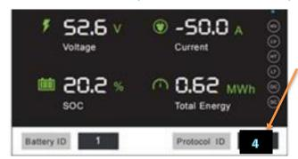
Protool ID is set to 4 for Victron GX using the front panel touchscreen.
