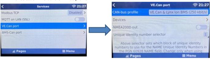
Then select VE.Can & CAN-bus BMS (250 kbit/s) and verify on main menu CAN-bus BMS battery data
