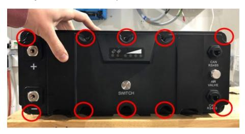
3. eFlex with serial number 2205## (made in May 2022 onward) contain a gasket lid, which can be easily removed after the screw removal.
