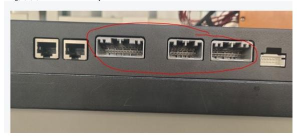
6. After  $\sim 60$  Mins: use multi-meter to read battery cell voltage from the plug. You will need fine/thin probe leads to analyze voltage in this manner.
