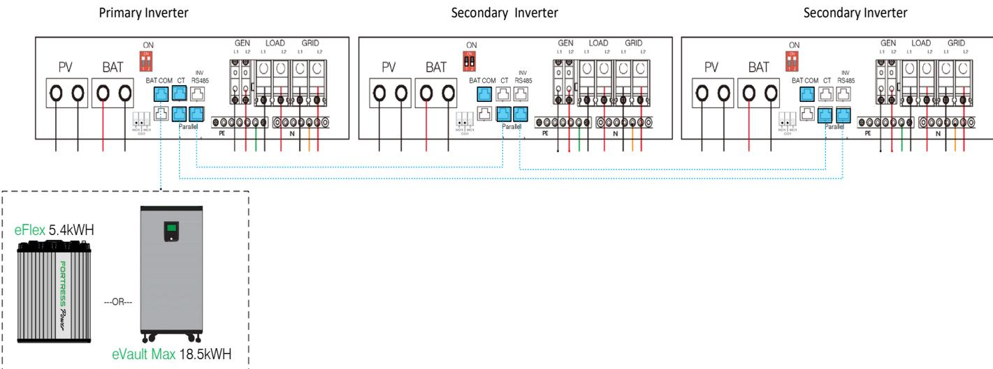
When paralleling multiple inverters, make sure to complete paralleling process by identifying which is the Primary inverter and the secondary on Parallel System area under the Advance Section. You can confirm by Selecting the Home Icon and view how many inverters are in connection (**PNUM**) and which **Role** each has (**P=Primary, S=Subordinate**)
