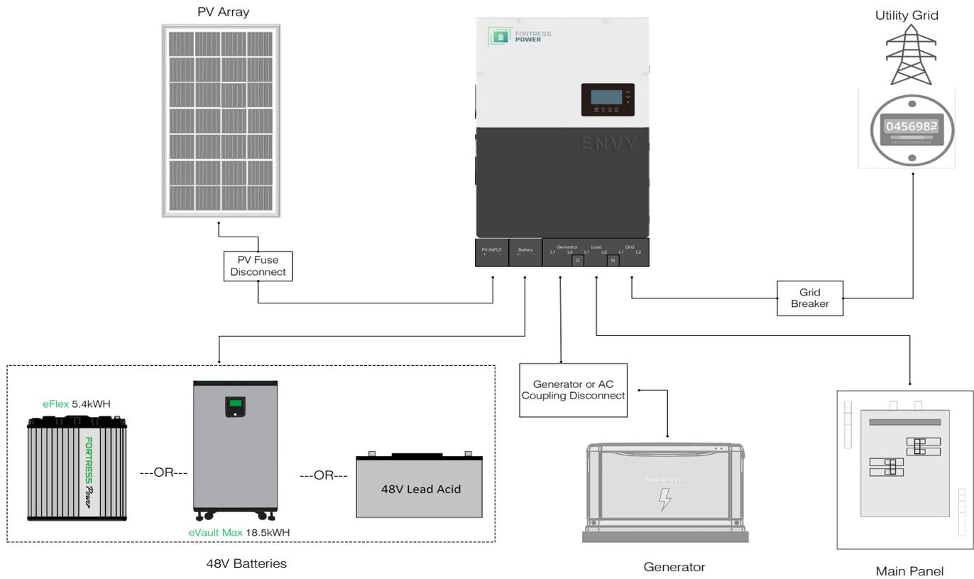
Please include the following recommended breakers for each system connection in accordance with the local jurisdiction. Battery breaker and Load breaker are already integrated in the Envoy inverter.
