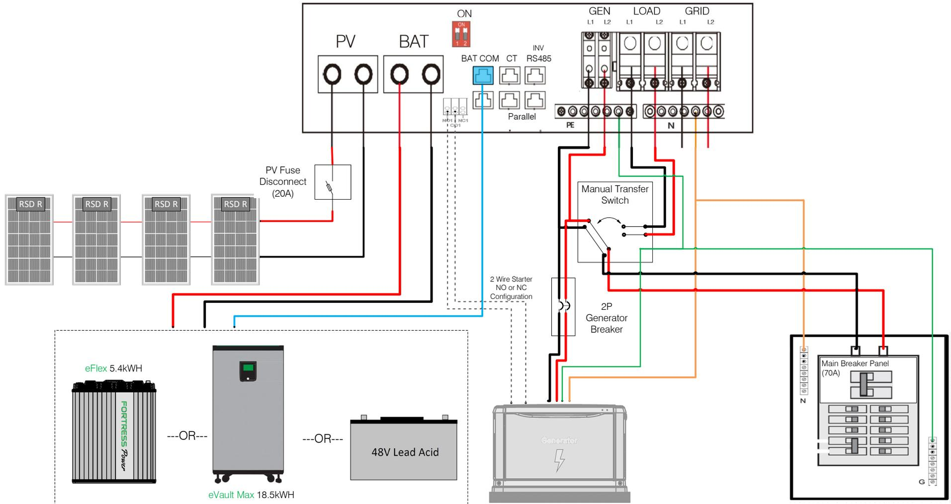
**WARNING: Make sure to turn off the Generator Breaker on the Envy before turning on the Generator and the PV system is bypassed. Fault or Damage will occur if power enters to the load side of the Envy.**
