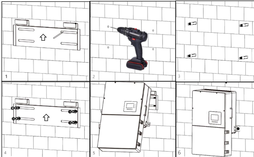
1. Mark the drill holes positions with the mounting bracket,
