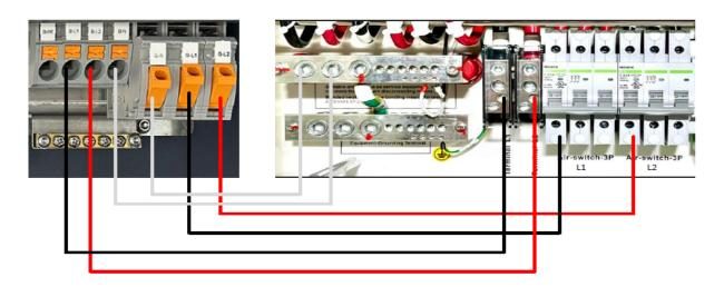
Figure 5.10 SEP to Inverter AC Wiring
