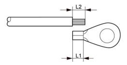
Figure 5.21 External Grounding Conductor Ring Terminal
