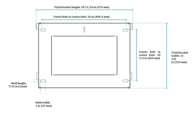
Figure 5.16 Inverter bracket dimensions
