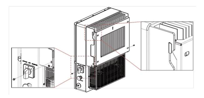
Figure 5.18 Inverter on mounting bracket and set screws
