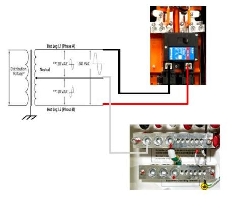
Figure 5.9 SEP Grid AC Wiring
