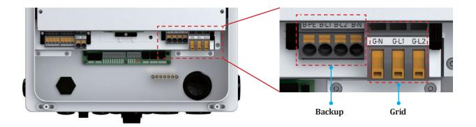
Figure 5.27 AC output terminals
