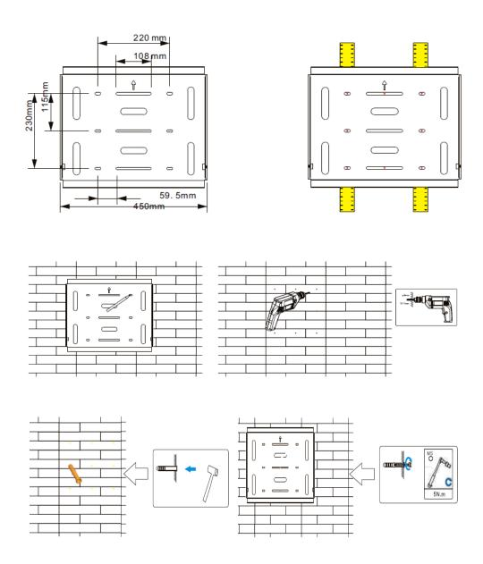
Figure 5.4 Install SEP Mounting Bracket
