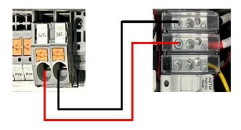
Figure 5.41 Battery Pack to Inverter Power Cable Connection
