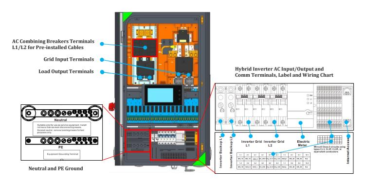
Figure 5.6 SEP Wiring Points
