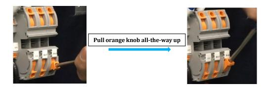
Figure 5.28 Grid AC Terminal Operation
