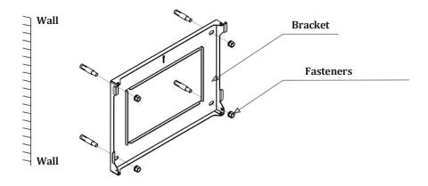
Figure 5.17 Fixing the bracket to the wall
