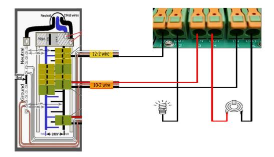
Figure 5.10 SEP to Load AC Wiring
