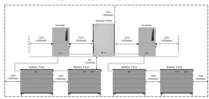
Figure 4.4 Avalon ESS Mounting Clearance
