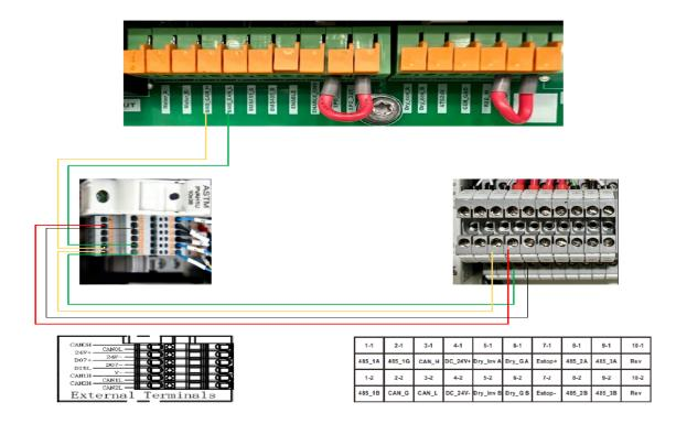
Figure 5.40 Battery Pack to Hybrid Inverter and SEP Communication Connection
