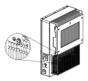
Figure 5.20 External Grounding Conductor Terminal Location
