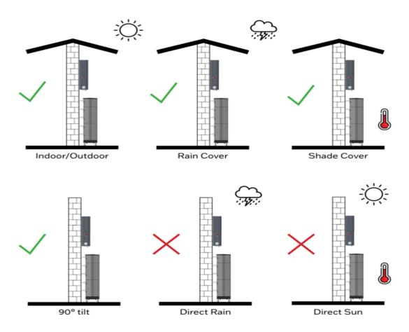
Figure 4.1 Recommended installation location
