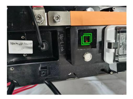
6. Once it is completed, the battery will make a beeping sound and reboot. You should see the SOC indicators. Remove Modbus tool cable and proceed with installation/commissioning process.
