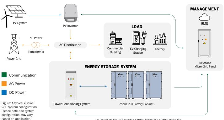
ESS includes: 125 kVA Inverter, battery, battery racks, BMS, HVAC, fire suppression, extraposition transformer, and outdoor rated enclosure
