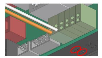
After completing the wiring, plug the other end of the Envy-to-Guardian cable into the INV485 port on the Envy inverter. Once connected, power on the Guardian and proceed with the commissioning process using the Guardian interface.
