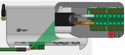
When setting up the Guardian with a Fortress Power Envy inverter, use the provided tworow, four-column connector to wire into the Guardian's communication port. For proper connection, refer to the cable pinout: connect the Orange/White wire to RS485 1A and the Orange wire to RS485 1B on the Guardian.
