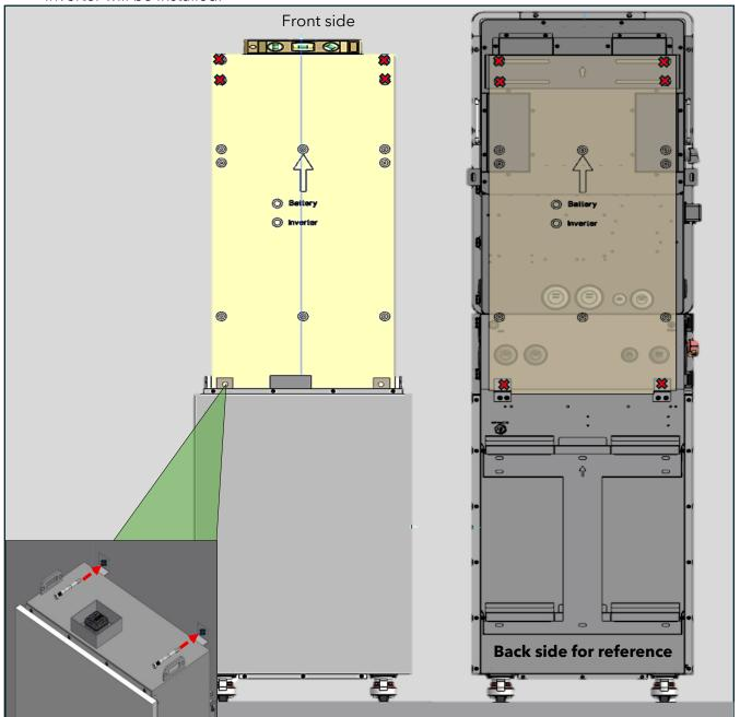
• Identify with an X the spot in which the mounting holes must be drilled. Remove the template and drill holes. If mounting on a concrete wall, use a drill with a masonry bit to create holes for anchors.
