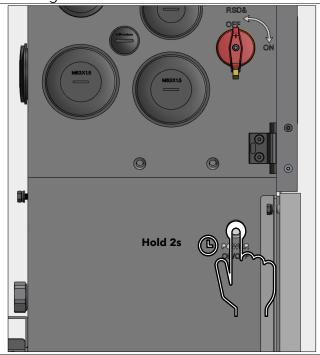
Once selected wait for less than 10seconds until the LED indicator returns to normal operation. You must do this while all batteries in the field.
